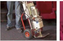
7. The 230V drive of the Movielift is mounted on a separate elevating truck and can be placed at a distance of maximum 10 m next to, in front of or behind the Movielift.
