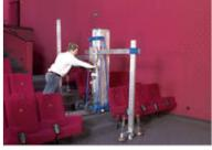
4. The Movielift can still be moved with the rollers even after the basic unit has been built up. Thus it is child's play to move it to each desired position in the particular row of seats.
